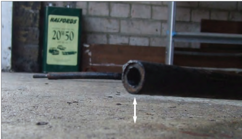
Picture 3: Bent anti-roll bar
